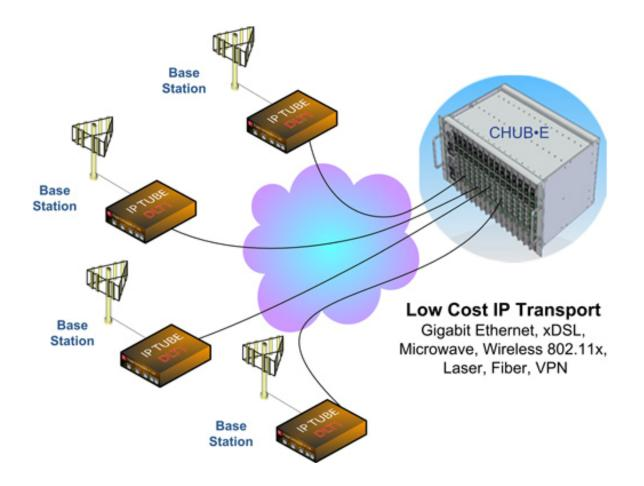
The Engage Communication IP•Tube is used to provide transparent interconnection of the base stations (BTSs), base station controllers (BSCs) and mobile switching centers (MSCs) over IP Ethernet packet-switched networks. The IP•Tube T1 maintains all the features of the cellular network BSC to BTS interconnections. Cellular phone service providers are able to save substantially by converting to a packet switch network from circuit TDM lease lines.
